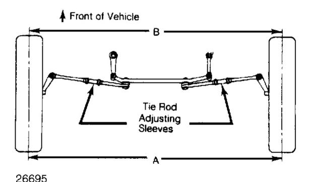
Fig. 2: Adjusting Tie Rod Sleeves (Top View)
