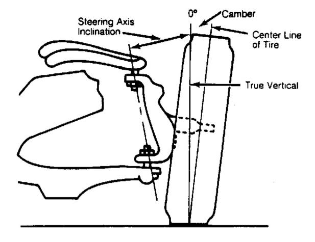
Fig. 6: Checking Steering Axis Inclination
